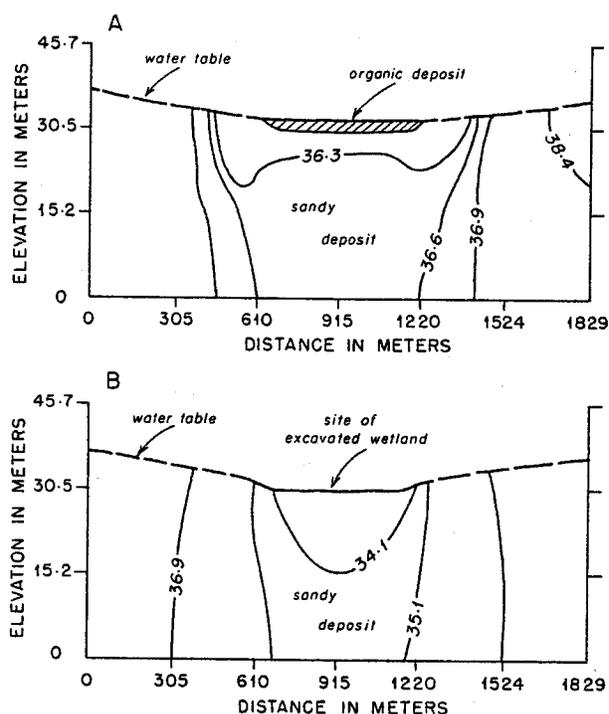
**Figure 3.** Head distribution in an ideal sand and gravel aquifer (A) with a wetland 1.5 m thick and (B) after organic deposits have been excavated. 36.3 and 34.1 represent lines of equal hydraulic potential, in meters above a standard datum. Vertical exaggeration: 20:1. (O'Brien 1987)
