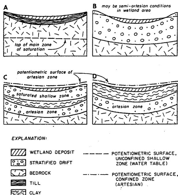
**Figure 2.** Diagrammatic cross-sections showing the relationship of wetlands to the principal zone of saturation (hydrologic position) for several geologic conditions. (A) Perched wetland. (B) Watertable wetland. (C) Watertable/artesian wetland. (D) Artesian wetland. (O'Brien and Motts 1980)
